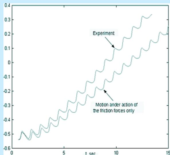
**Experimental Data:** A comparison of inertial versus frictional acceleration for the gyroscope.
